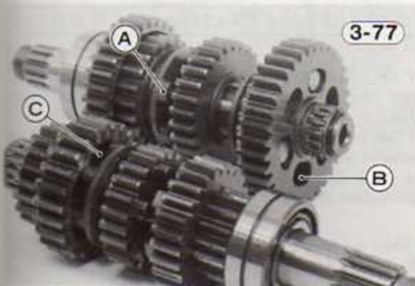
A. Gear Dog B. Dog Hole C. Dog Recess
