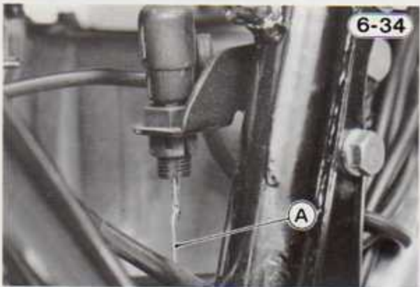
A. Rear Brake Light Switch Spring
