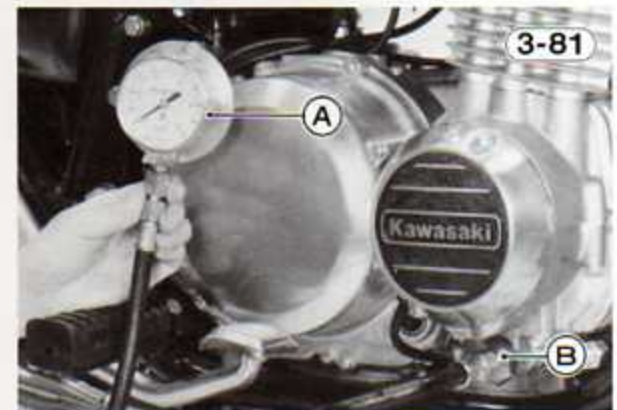
A. Oil Pressure Gauge: 57001-164 B. Adapter: 57001-403
