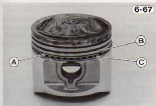
A. Oil Ring Expander B. Upper Steel Rail C. Lower Steel Rail
