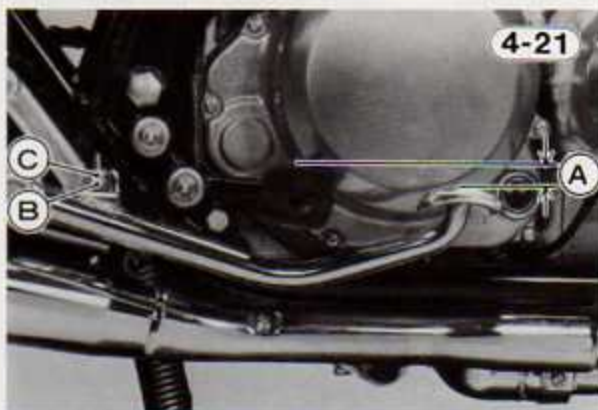
A. 0 – 30 mm B. Adjusting Bolt C. Locknut
