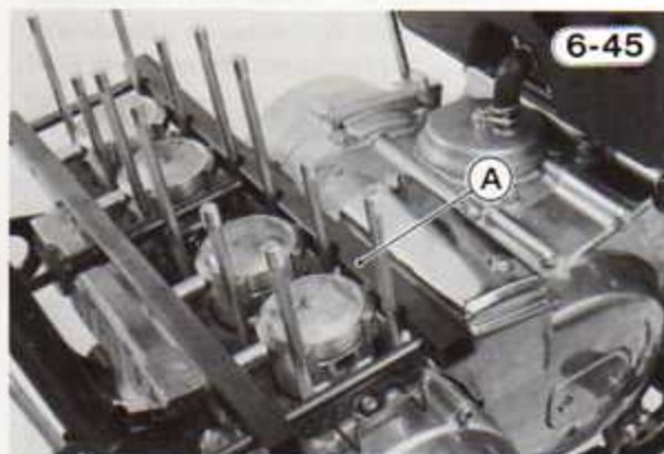
A. Piston Ring Compressor: 57001-531
