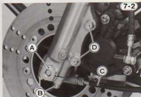
A. Axle Nut B. Axle Clamp Nuts
