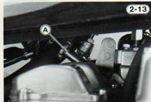
A. Idle Adjusting Screw
